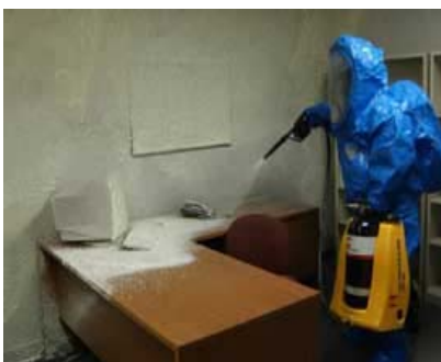
The Intelagard Macaw is a man-portable compressed air foam backpack system
